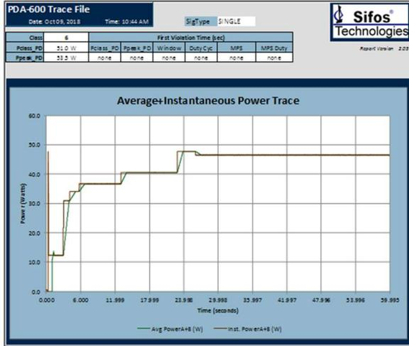
Figure 8: Streaming Power Trace from Class 6 PD
