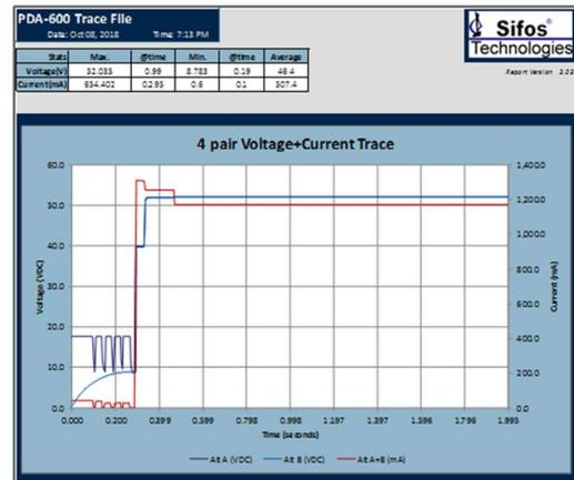
Figure 4: Class 8 PD Power-Up V+I Waveform
