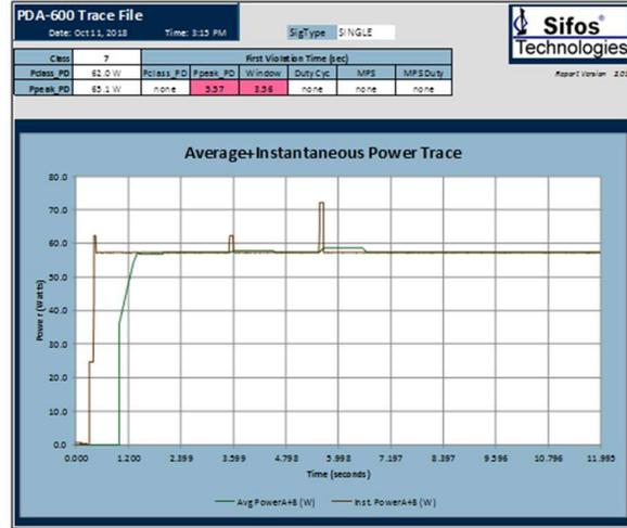
Figure 9: Streaming Power Trace from Class 7 PD
