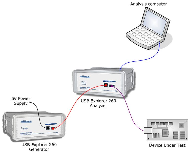
As the Explorer 260 Generator is powered by the USB bus, the power supply for the Device Under Test must be supplied by an external power supply on the B connector of the Generator, as displayed in the figure above.
