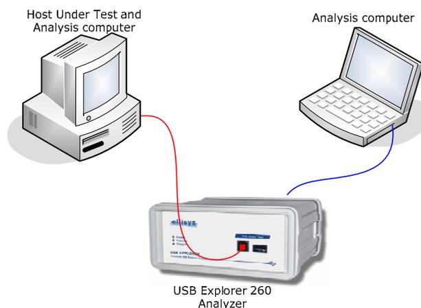
Figure 1 - Configuration with two separate computers
