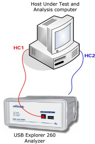
Figure 2 - Configuration with only one computer
