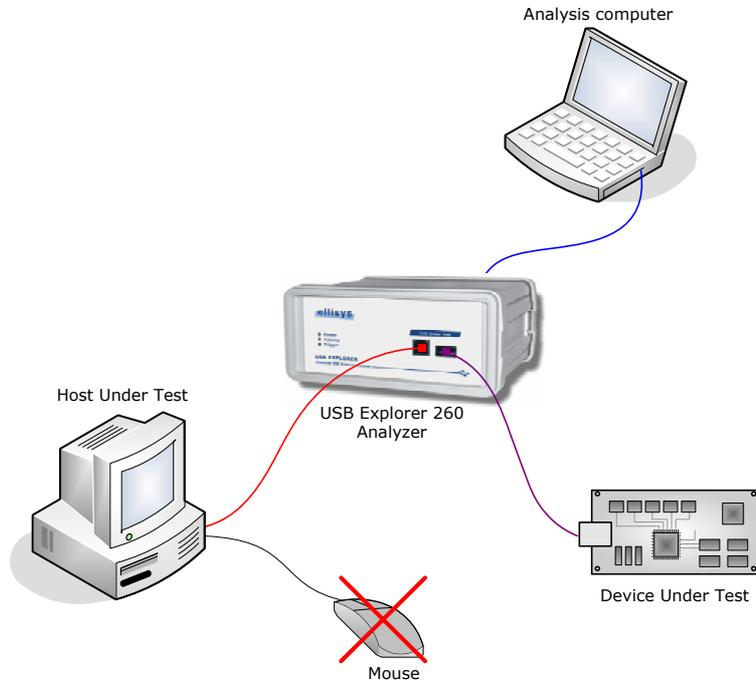
**Figure 4 - Wrong connection with more than one DUT**
