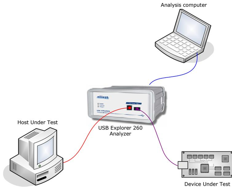
**Figure 3 - Connecting only one Device Under Test**
