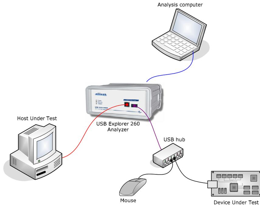
**Figure 5 - Correct connection with more than one DUT using a Hub**
