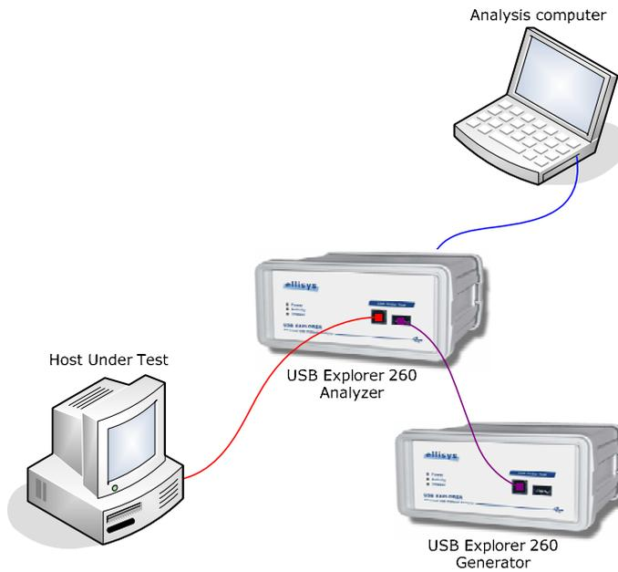
**Connecting the Generator for Inline Error Injection**
